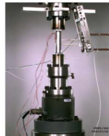
b) SNTT fracture test setup
