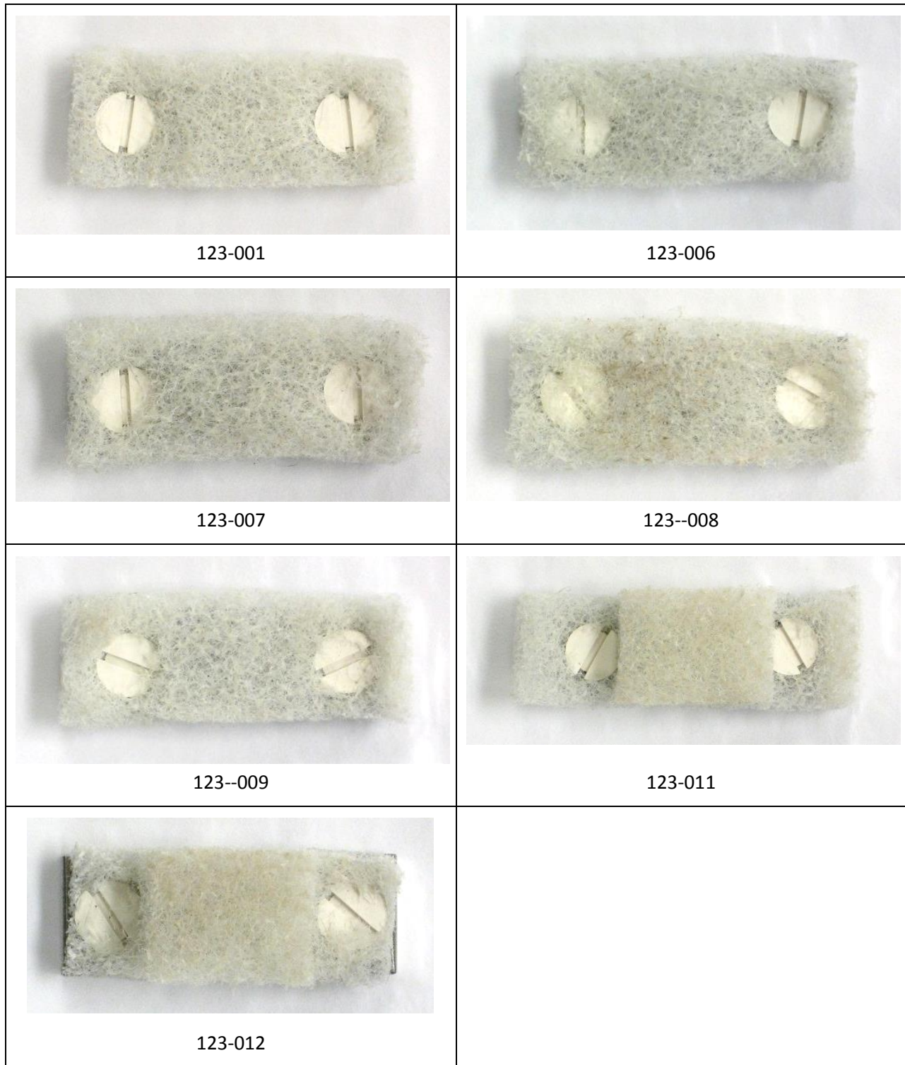
Figure 8. Dry pad samples collected from canister MPC-123, Diablo Canyon.
