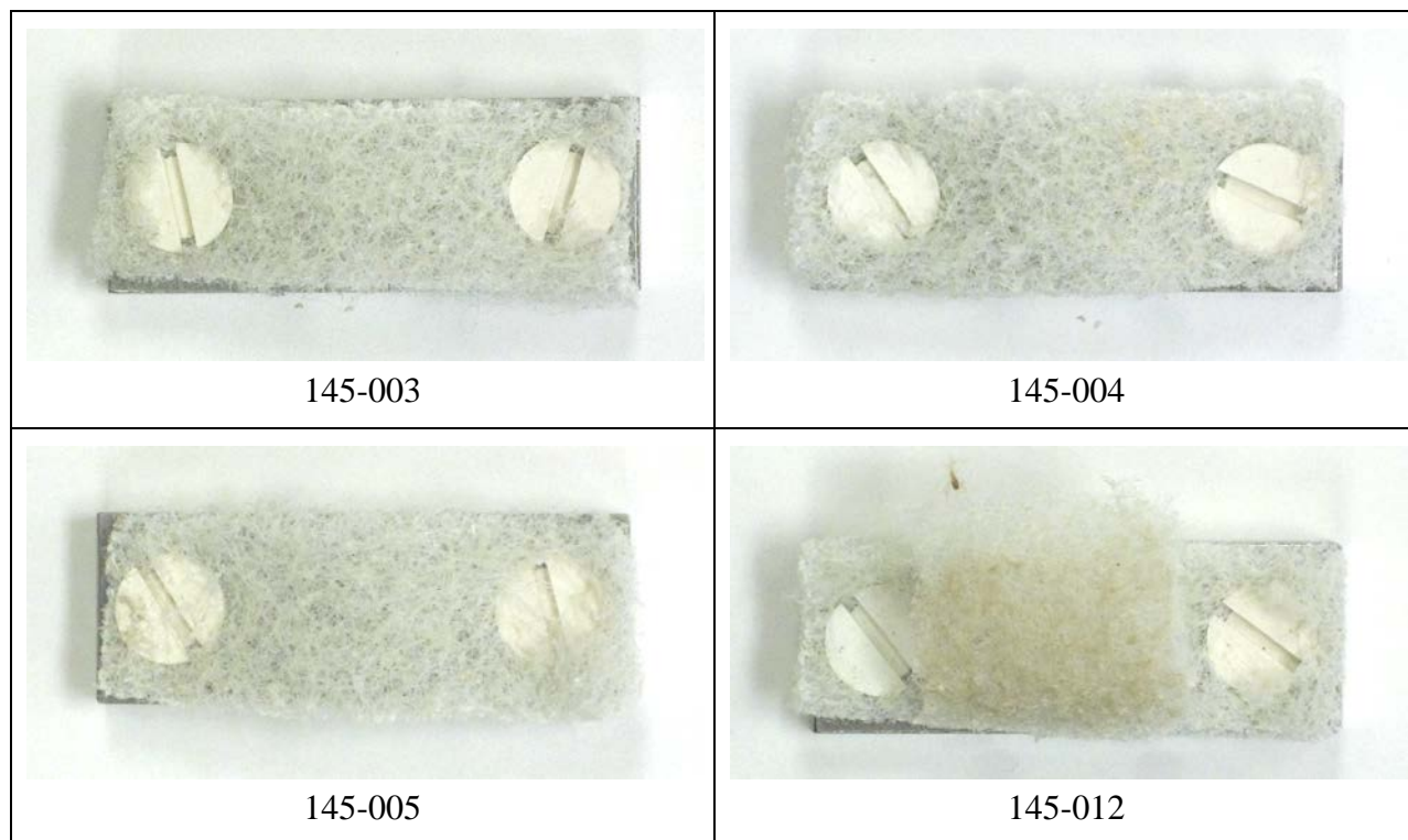
Figure 6. Dry pad samples collected from canister MPC-145, Hope Creek. Note the small seed adhering to the upper edge of sample 145-012.
