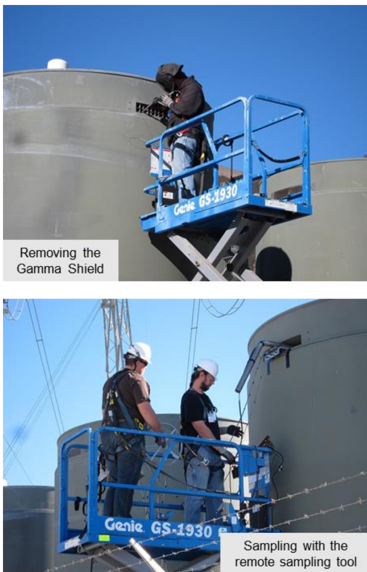
Figure 2. Sampling dust from the surface of interim storage canisters within their overpacks.
