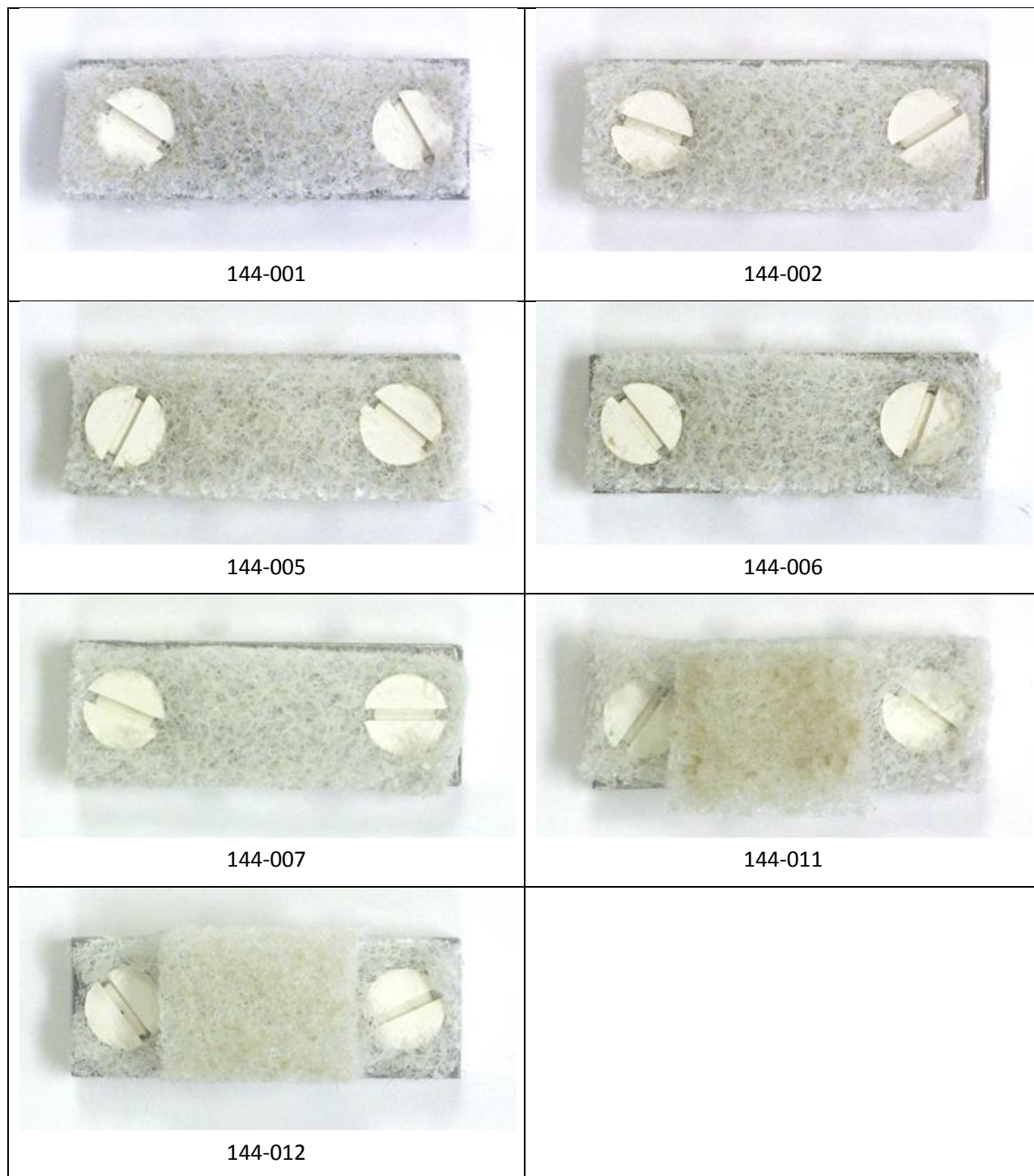
Figure 4. Dry pad samples collected from canister MPC-144, Hope Creek.
