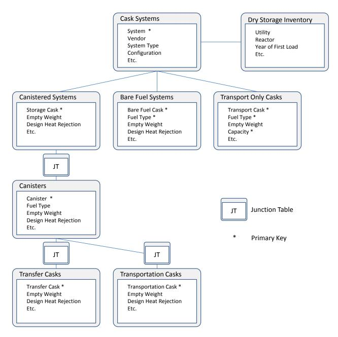
Figure 3.2-1 Dry Storage Cask/Inventory Database Structure
