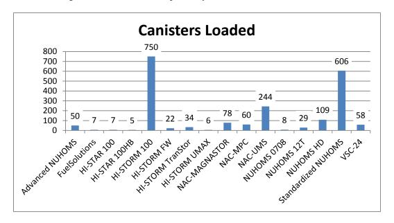
Figure 4.2-1 Distribution of Canisters Loaded Versus Canistered Storage Systems
