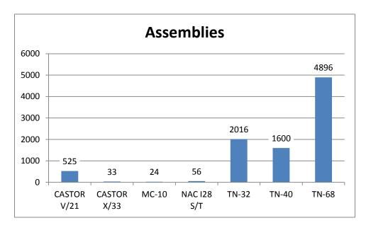
Figure 4.1-2 Distribution of Assemblies Versus Bare Fuel Storage Systems
