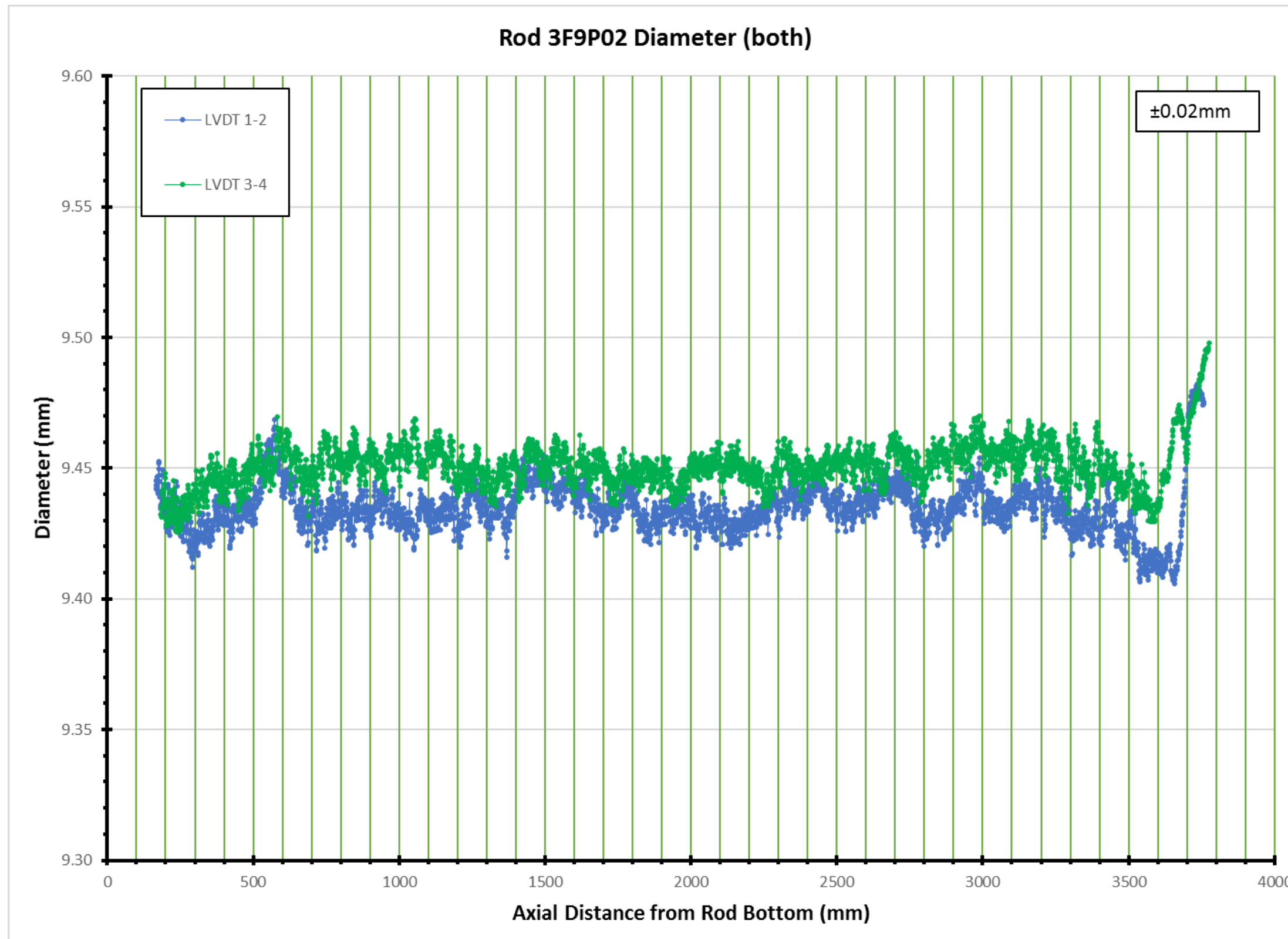
Figure A.7. Rod 3F9P02 LVDT Diameter Measurements.
