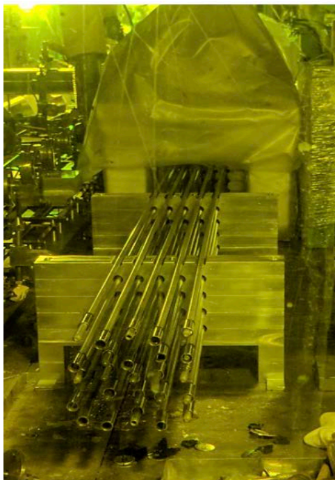
Figure 34. Set Up for Measuring a 5 \times 5 Array of 25 Full-Length Spent Fuel Rods Using a Fork Detector at ORNL's IFEL Hot Cell with All Locations Filled with Sister Rods (Left) and with 8 Partially Vacant Locations (Right).
