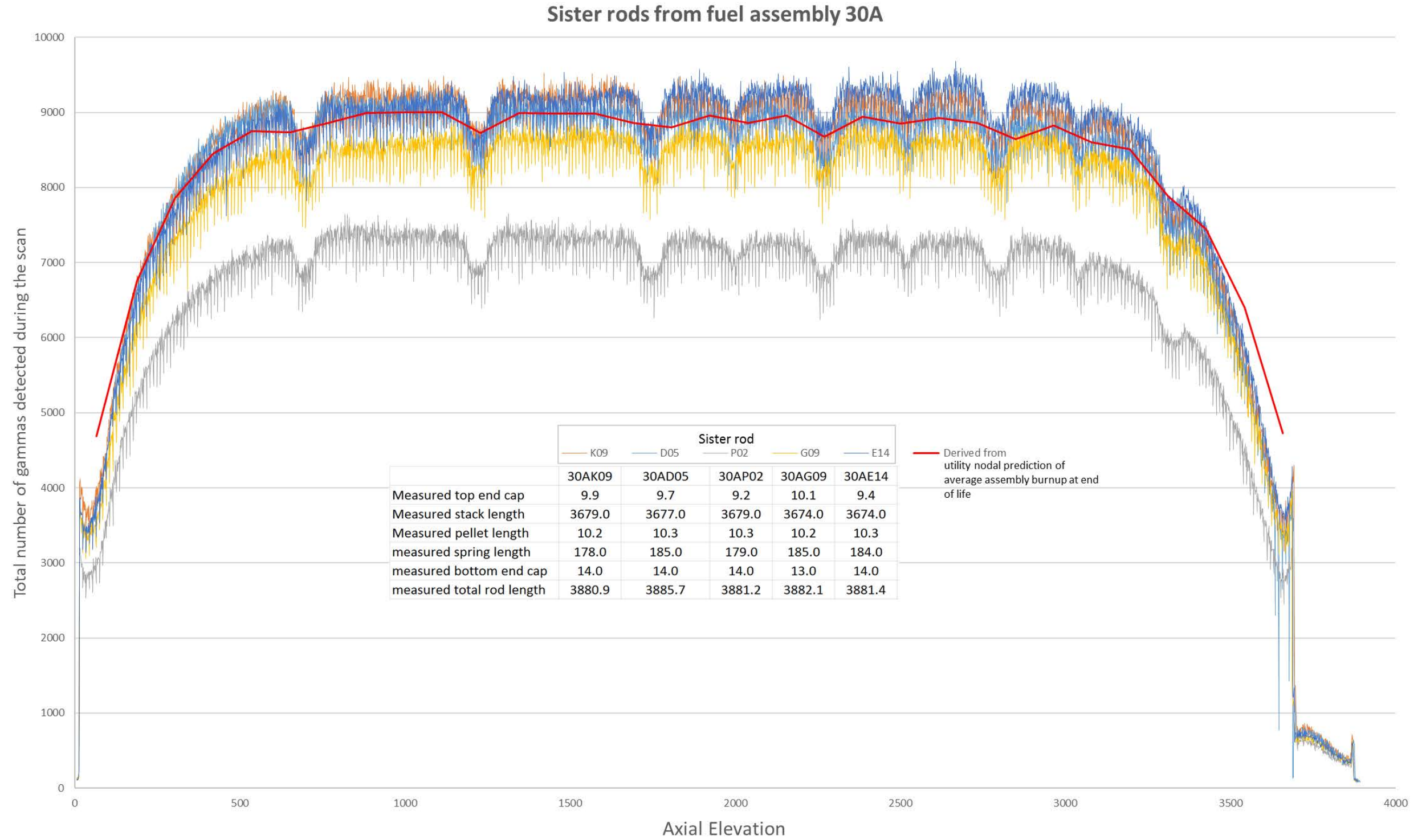
Figure 16. Gamma Scans for Sister Rod from Fuel Assembly 30A.
