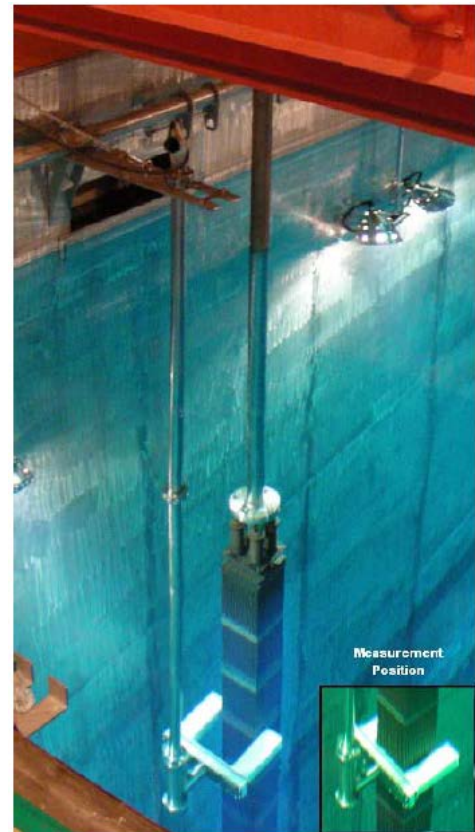
Figure 31. Measurement of a Spent Fuel Assembly in a Pool Using a Fork Detector [8].
