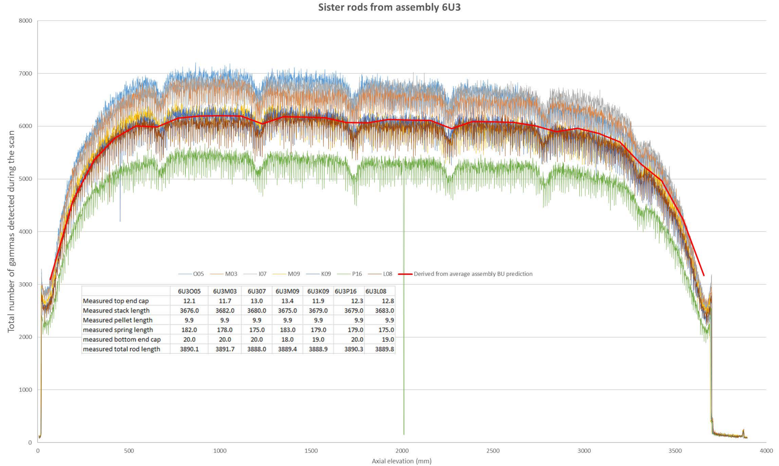
Figure 22. Gamma Scans for Sister Rod from Fuel Assembly 6U3.
