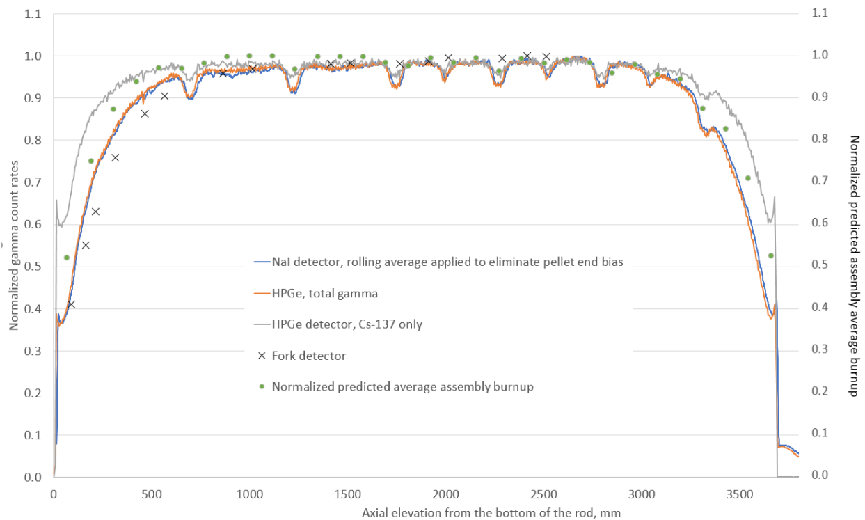
Figure 15. Comparison of Gamma Count Rates Collected by Three Different Detectors for Sister Rod 30AE14: HPGe, fork, and NaI. The Normalized Predicted Average Assembly Axial Fuel Burnup is also Plotted for Reference.
