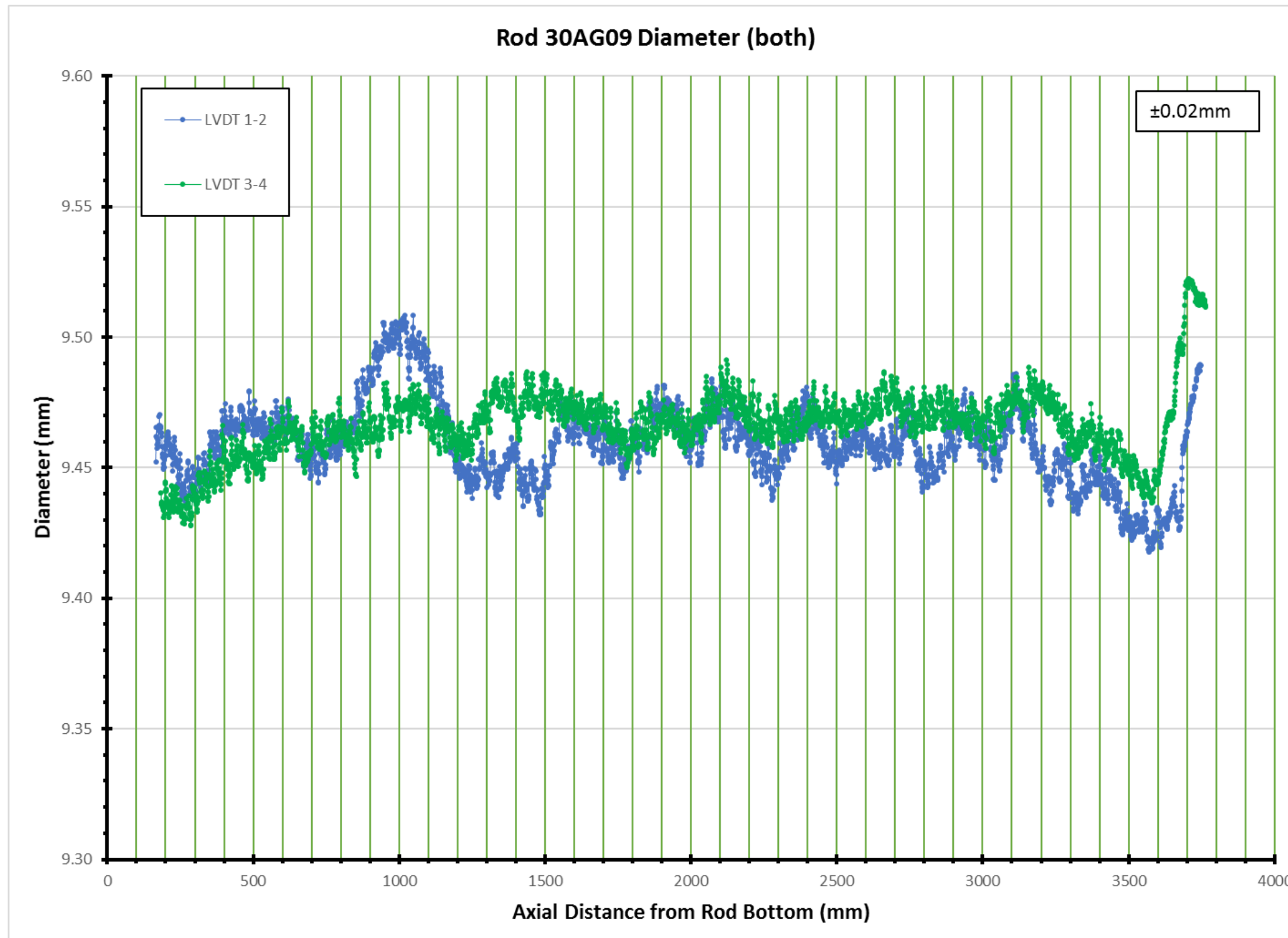
Figure A.21. Rod 30AG09 LVDT Diameter Measurements.
