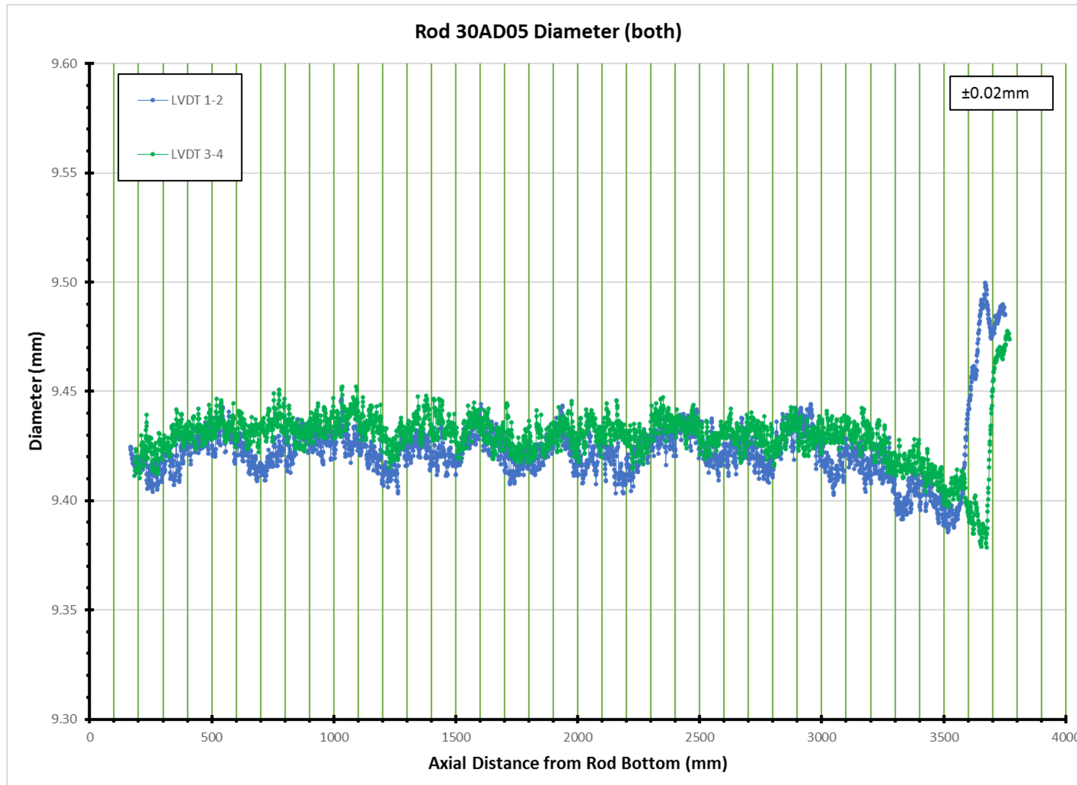
Figure A.191 Rod 30AD05 LVDT Diameter Measurements.
