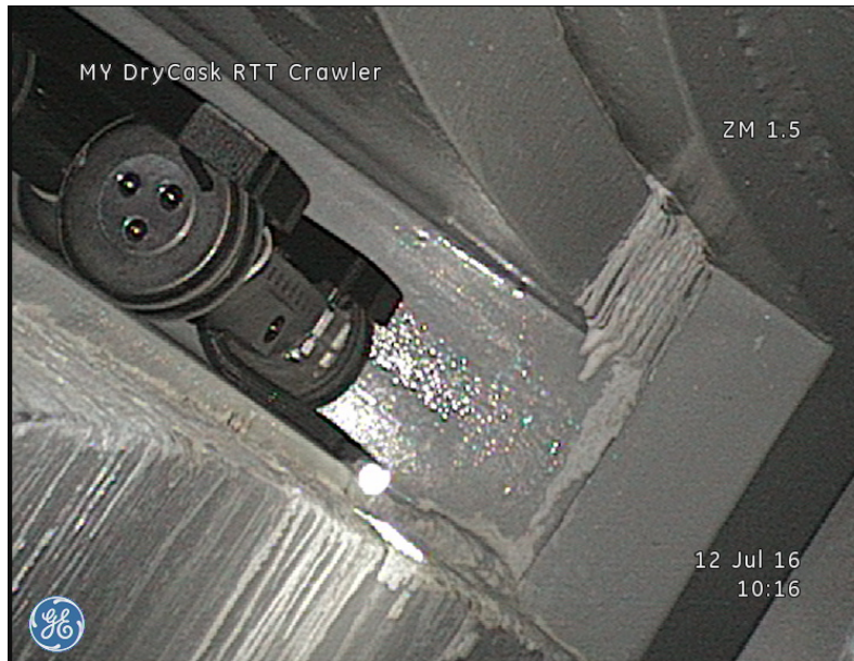
Figure 12. Video image of white crusts of cementitious material on the inner surface of the overpack, located near an outlet vent.
