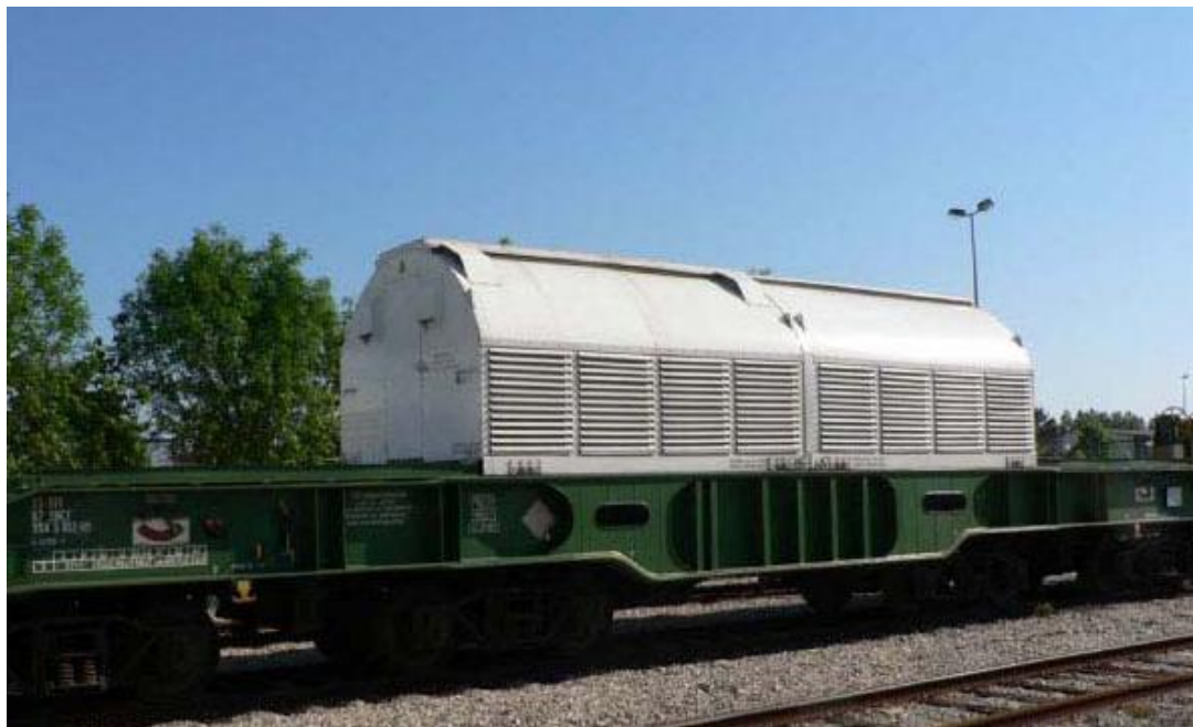
Figure 2.7 Rail Cask with Personnel Barrier Loaded on a Rail Car [DOE 2008c]
