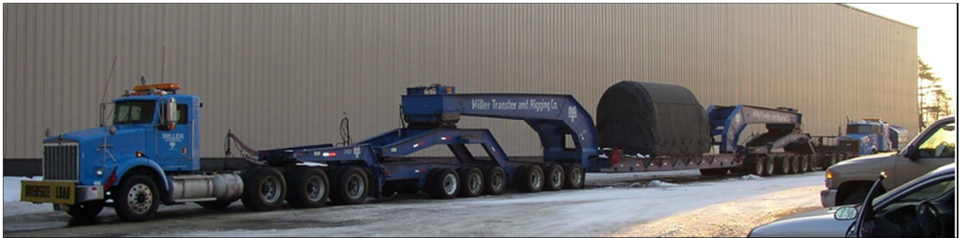
An Empty Transnuclear TN-32 Cask is Transported on a Miller Transport Heavy-Haul Tractor-Trailer
