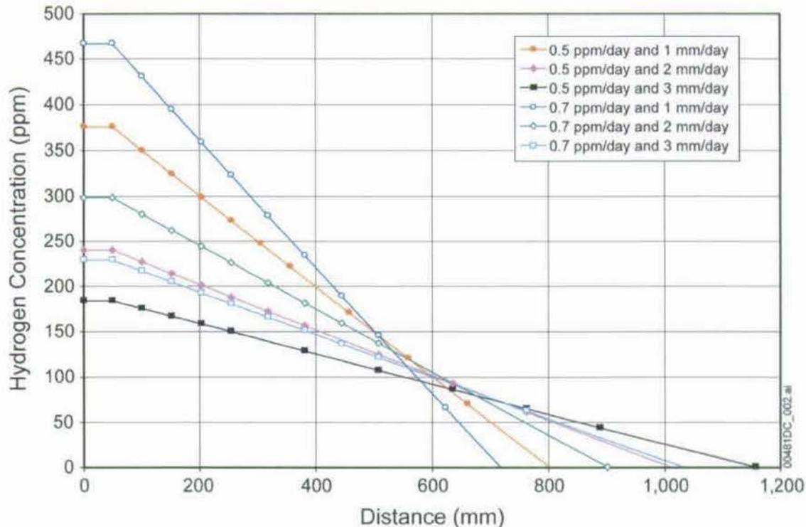
Figure 7. Hydrogen Concentration in Drip Shield Versus Distance from Contact Area
