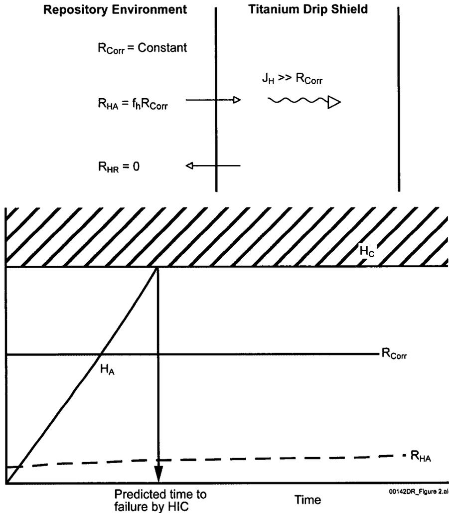
NOTE: This schematic shows hydrogen absorption during passive general corrosion of titanium (refers to the mathematical model described in Section 6.1.5)
