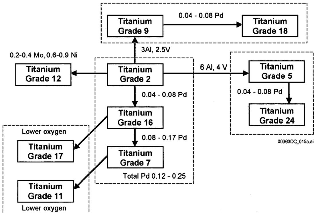
NOTE: Alloys grouped by the dotted lines have same mechanical properties, regardless of the chemical compositions (amount of Pd).
