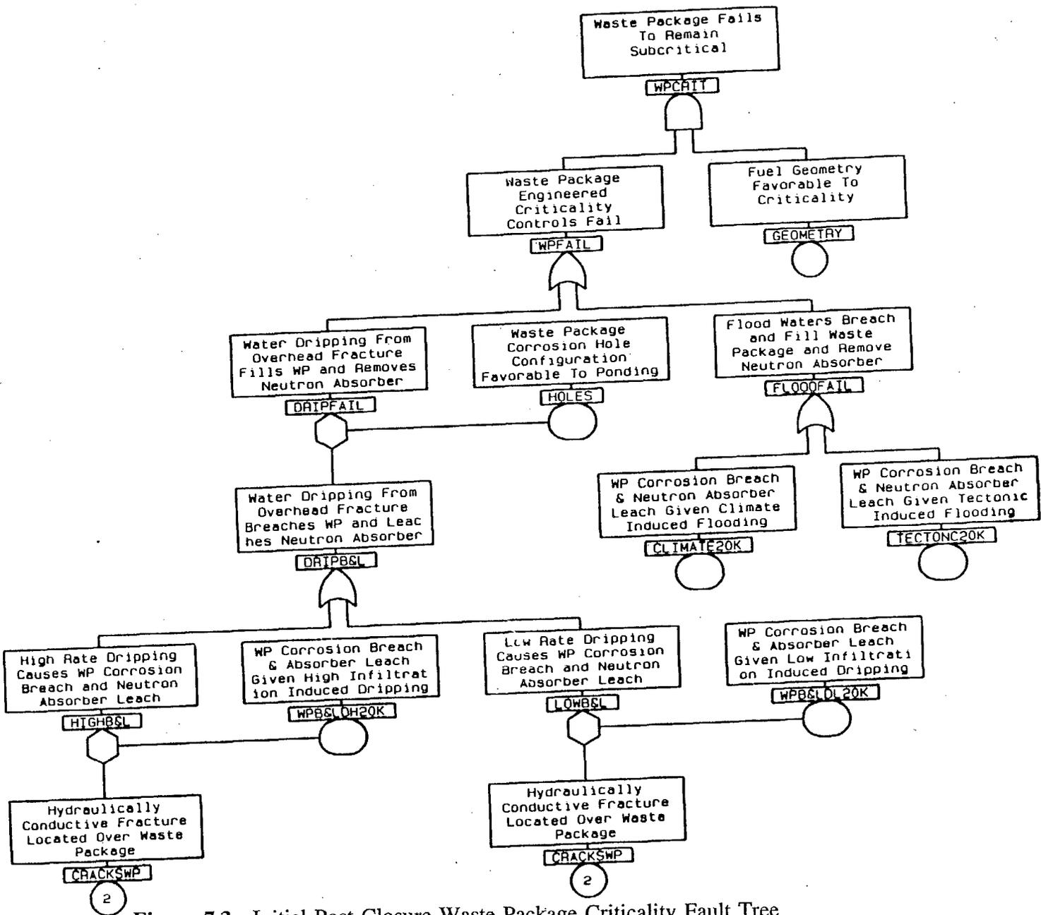
Figure 7.3. Initial Post-Closure Waste Package Criticality Fault Tree
