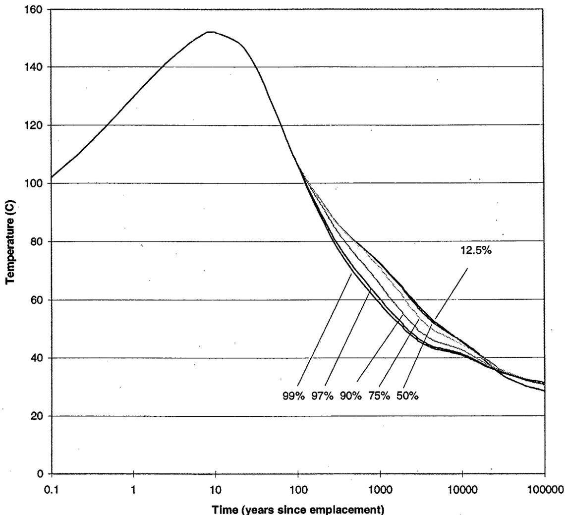
Figure 7.7. Waste Package surface temperature as a function of time for a mass loading of 6.0 kg U/m<sup>2</sup> (approximately 24 MTU/acre), curves are for different locations in the repository (0% - center, 25% - mid-way from center to edge, 100% - edge)
