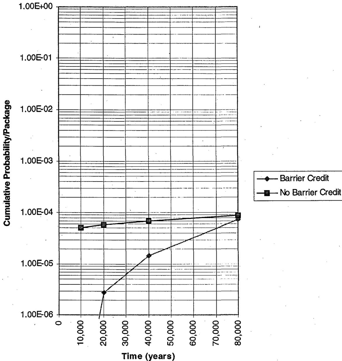
Figure 7.15. Cumulative per-package criticality probability for various times since emplacement with and without credit for the waste package barriers (TBV).
