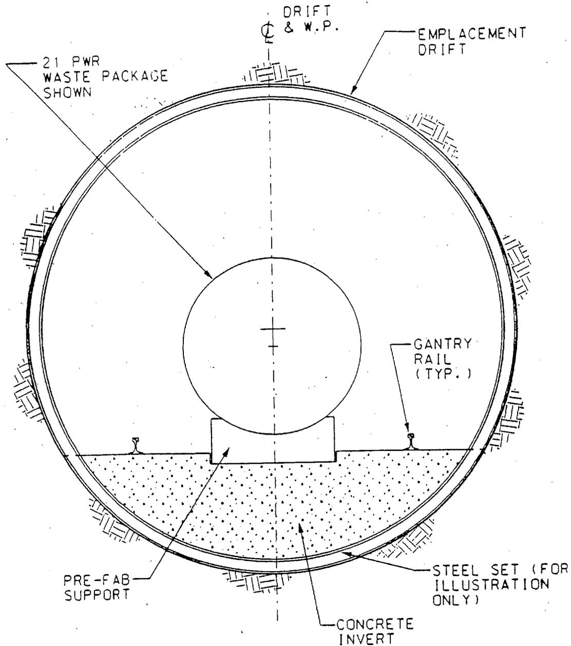
Figure 7.1. Waste Package and Local Drift Environment
