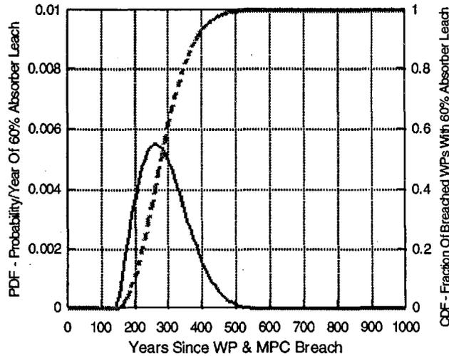
Figure 7.12. Distribution of time to leach 60% of neutron absorbing material from MPC-WP basket structure exposed to continuously wetted conditions.
