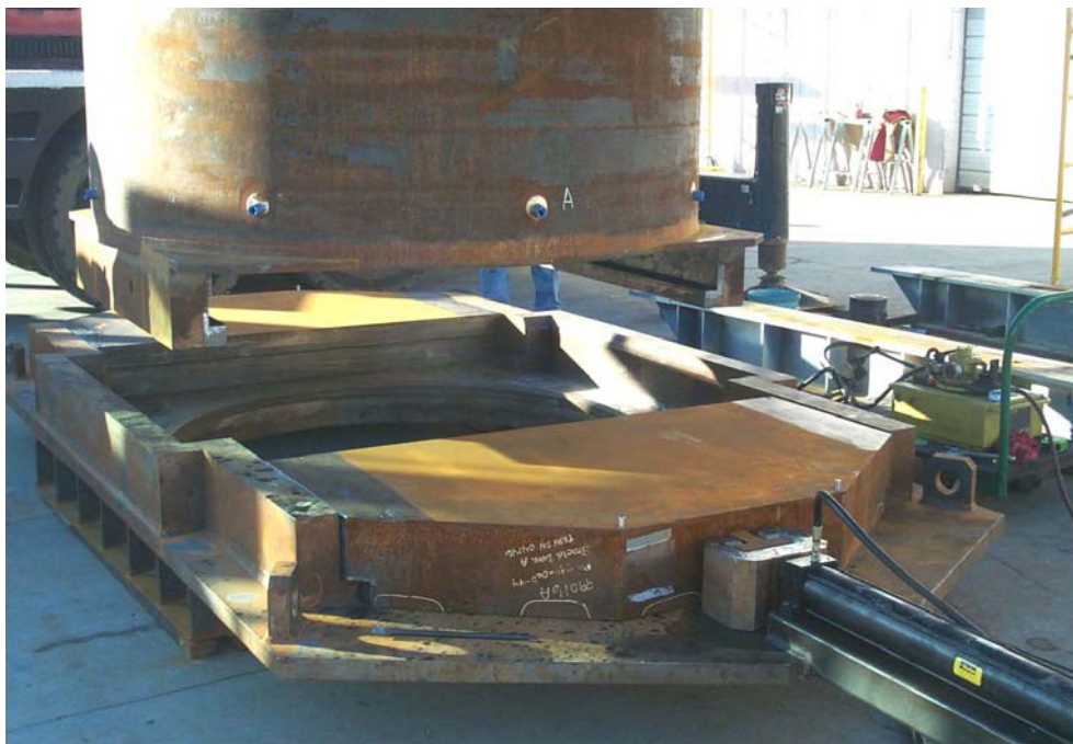
Figure 5-3 NAC Adaptor Plate Door Operation (NAC SNFDS Seminar)
