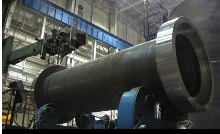
HI-STAR 60 Containment and Top/Bottom Forgings during Fabrication at the Holtec Manufacturing Division
