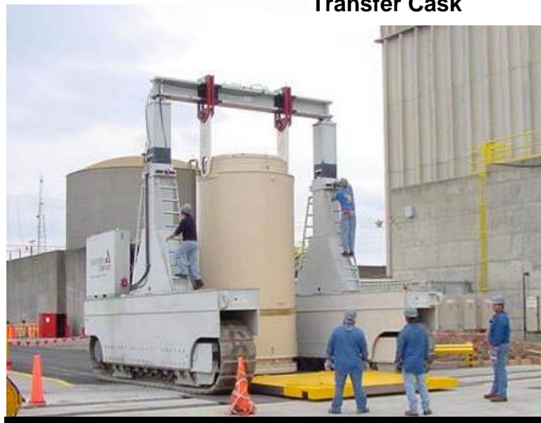
125 Ton HI-TRAC Transfer Cask and Transporter
