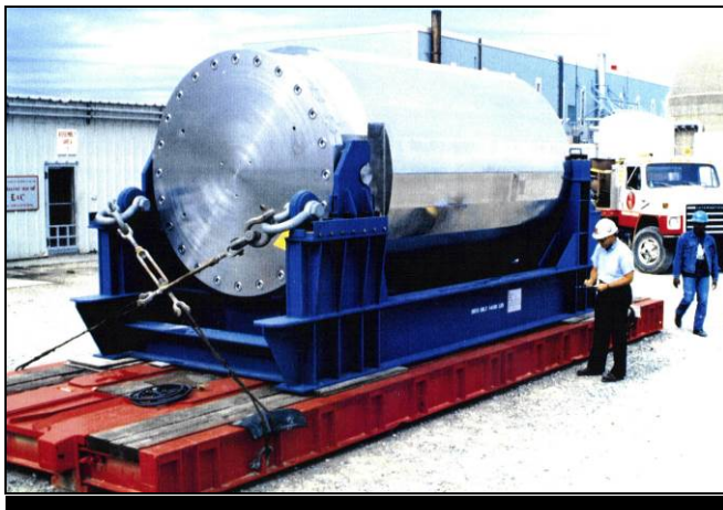
NAC I28 S/T Used Fuel Storage Cask
