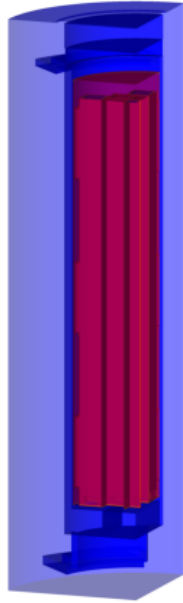
Figure A1-2 Sectional view of the Sierra Nuclear Corporation's ventilated vertical concrete storage cask-17 dry storage system used in computation
