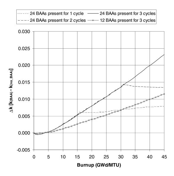
Figure 21  $\Delta k$  values as a function of burnup for Westinghouse 17 × 17 fuel with 4.0 wt %  $^{235}$ U initial enrichment that has been exposed to Westinghouse Pyrex BAA rods (3 cycles of 15 GWd/MTU per cycle were assumed)
