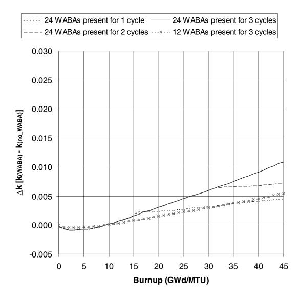
Figure 8  $\Delta k$  values as a function of burnup for Westinghouse 17  $\times$  17 fuel with 5.0 wt %  $^{235}$ U initial enrichment that has been exposed to Westinghouse WABA rods (3 cycles of 15 GWd/MTU per cycle were assumed)
