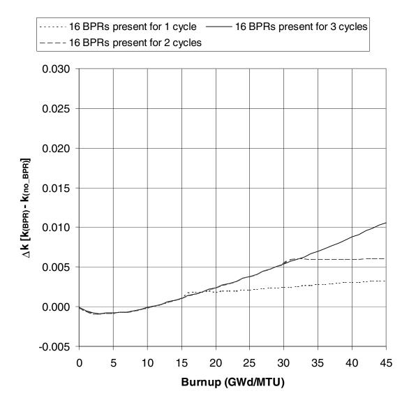
Figure 25  $\Delta k$  values as a function of burnup for B&W 15  $\times$  15 fuel with 5.0 wt %  $^{235}$ U initial enrichment that has been exposed to B&W (2.0 wt % B<sub>4</sub>C) BPRs (3 cycles of 15 GWd/MTU per cycle were assumed)
