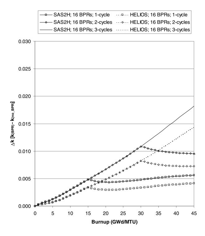
Figure 37 Comparison of reactivity differences ( $\Delta k$  values relative to the no BPR condition) as calculated with CSAS1X based on isotopics calculated with SAS2H and HELIOS for actinide-only burnup credit. The results correspond to B&W 15  $\times$  15 fuel with 4.0 wt %  $^{235}$ U initial enrichment that has been exposed to 16 B&W BPRs.
