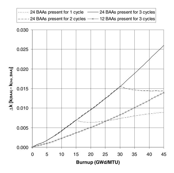
Figure 32  $\Delta k$  values as a function of burnup for Westinghouse 17  $\times$  17 fuel with 4.0 wt %  $^{235}$ U initial enrichment that has been exposed to Westinghouse BAA rods (3 cycles of 15 GWd/MTU per cycle were assumed). The results are based on SAS2H-depletion and CSAS1X-criticality calculations with "actinide-only" nuclides (See Table 8 for specific nuclides).
