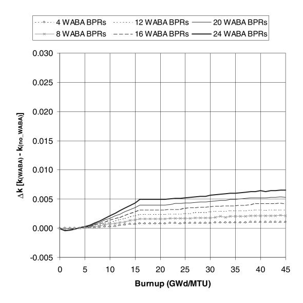
Figure 14  $\Delta k$  values as a function of burnup for Westinghouse 17  $\times$  17 fuel with 4.0 wt %  $^{235}$ U initial enrichment that has been exposed to various numbers of Westinghouse WABA rods for the first 15 GWd/MTU of burnup
