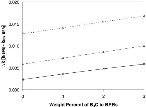
Figure 28  $\Delta k$  values for B&W 15  $\times$  15 fuel with 4.0 wt %  $^{235}$ U initial enrichment and a total burnup of 45 GWd/MTU that has been exposed to BPRs with varying poison loading and burnup exposures
