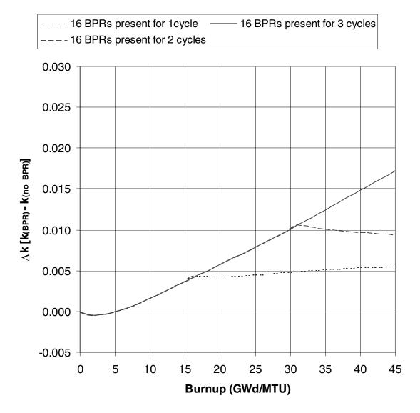
Figure 33  $\Delta k$  values as a function of burnup for B&W 15  $\times$  15 fuel with 4.0 wt  $\%^{235}$ U initial enrichment that has been exposed to B&W (2.0 wt % B<sub>4</sub>C) BPRs (3 cycles of 15 GWd/MTU per cycle were assumed). The results are based on SAS2H-depletion and CSAS1X-criticality calculations with "actinide + fission product" nuclides (See Table 8 for specific nuclides).
