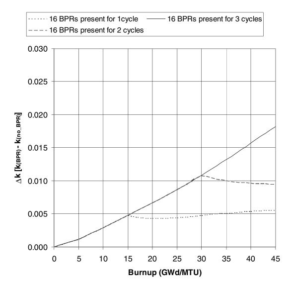
Figure 34  $\Delta k$  values as a function of burnup for B&W 15  $\times$  15 fuel with 4.0 wt %  $^{235}$ U initial enrichment that has been exposed to B&W (2.0 wt % B<sub>4</sub>C) BPRs (3 cycles of 15 GWd/MTU per cycle were assumed). The results are based on SAS2H-depletion and CSAS1X-criticality calculations with "actinide-only" nuclides (See Table 8 for specific nuclides).
