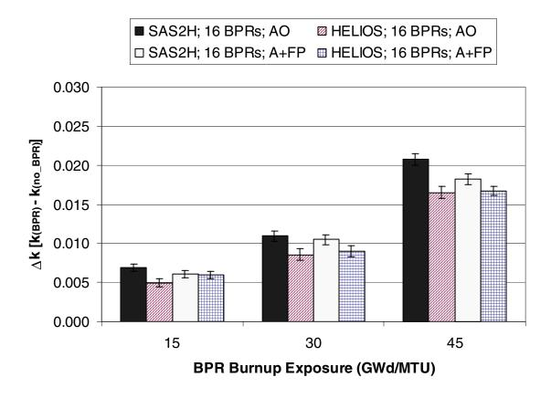
Figure 40 Comparison of reactivity differences ( $\Delta k$  values relative to the no BPR condition) in the GBC-32 cask (45 GWd/MTU, 5-year cooling) as calculated with KENO V.a for actinide-only (AO) and actinide + fission product (A + FP) burnup credit, based on isotopic compositions from SAS2H and HELIOS depletion calculations. The results correspond to fuel with 4.0 wt  $\%^{235}$ U initial enrichment that has been exposed to 24 B&W (2 wt % B<sub>4</sub>C) BPRs for various burnups.
