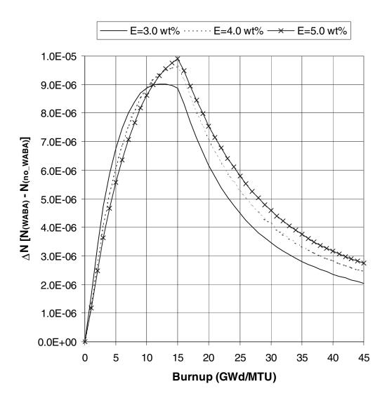
Figure 12 Differences in  $^{239}$ Pu atom densities,  $\Delta N$  values, as a function of burnup for Westinghouse 17  $\times$  17 fuel with various initial enrichments that have been exposed to 24 Westinghouse WABA rods for the first 15 GWd/MTU of burnup
