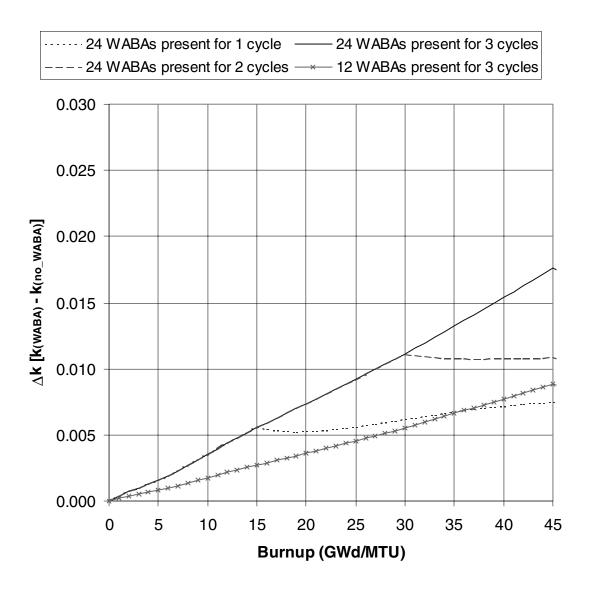
Figure 30  $\Delta k$  values as a function of burnup for Westinghouse 17  $\times$  17 fuel with 4.0 wt %  $^{235}$ U initial enrichment that has been exposed to Westinghouse WABA rods (3 cycles of 15 GWd/MTU per cycle were assumed). The results are based on SAS2H-depletion and CSAS1X-criticality calculations with "actinide-only" nuclides (See Table 8 for specific nuclides).
