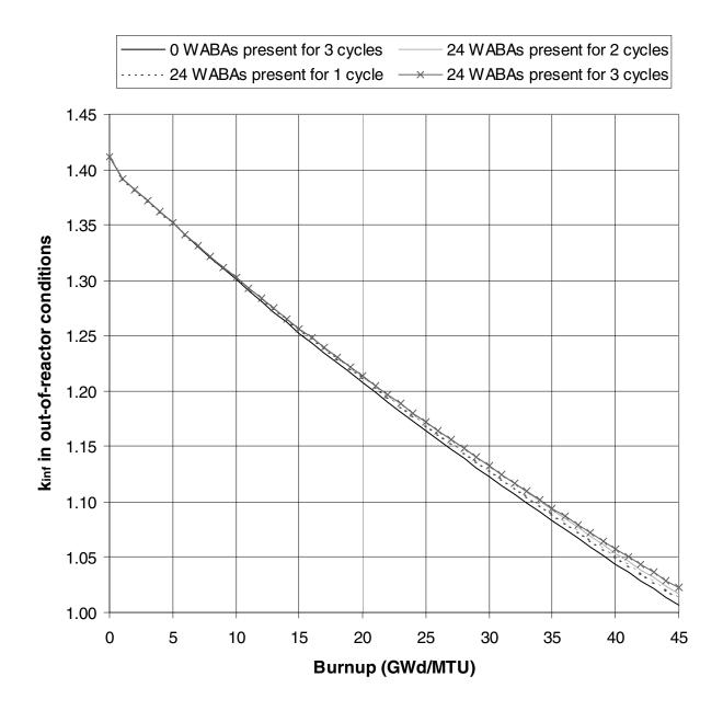
Figure 5  $k_{inf}$  values as a function of burnup for various WABA exposures. The results correspond to fuel with 4.0 wt %  $^{235}$ U initial enrichment that has been exposed to Westinghouse WABA rods (3 cycles of 15 GWd/MTU per cycle were assumed).
