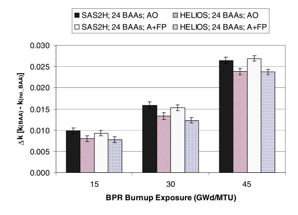
Figure 39 Comparison of reactivity differences ( $\Delta k$  values relative to the no BPR condition) in the GBC-32 cask (45 GWd/MTU, 5-year cooling) as calculated with KENO V.a for actinide-only (AO) and actinide + fission product (A + FP) burnup credit, based on isotopic compositions from SAS2H and HELIOS depletion calculations. The results correspond to fuel with 4.0 wt % <sup>235</sup>U initial enrichment that has been exposed to 24 BAA BPRs for various burnups.
