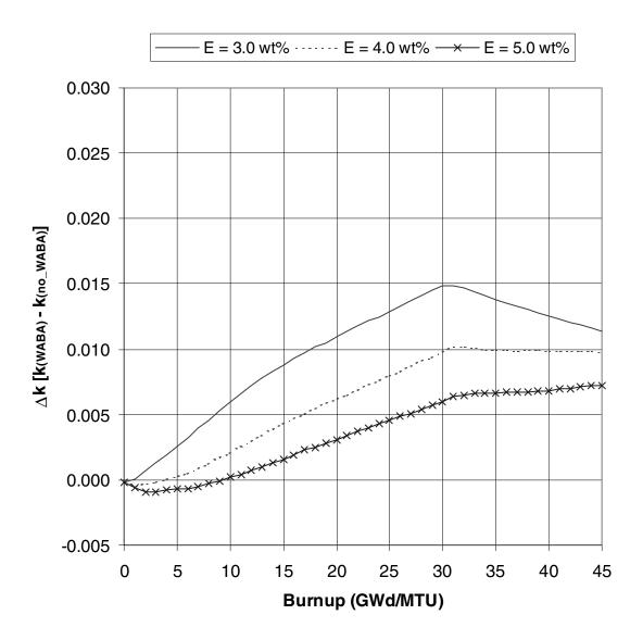
Figure 10  $\Delta k$  values as a function of burnup for Westinghouse 17  $\times$  17 fuel with various initial enrichments that have been exposed to 24 Westinghouse WABA rods for the first 30 GWd/MTU of burnup
