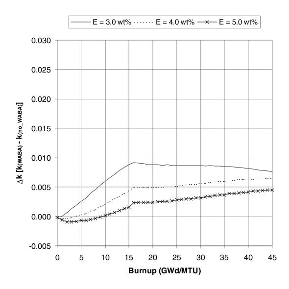
Figure 9  $\Delta k$  values as a function of burnup for Westinghouse 17  $\times$  17 fuel assemblies with various initial enrichments that have been exposed to 24 Westinghouse WABA rods for the first 15 GWd/MTU of burnup
