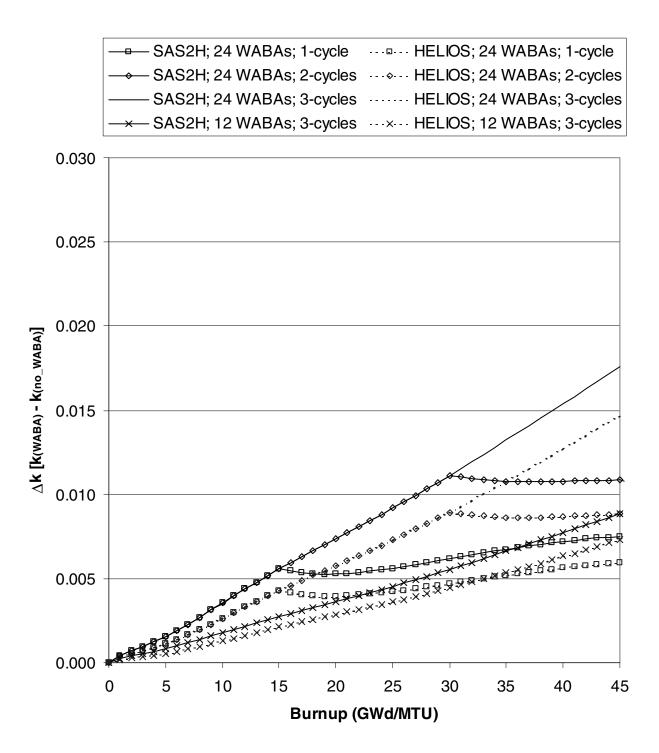
Figure 35 Comparison of reactivity differences ( $\Delta k$  values relative to the no BPR condition) as calculated with CSAS1X based on isotopics calculated with SAS2H and HELIOS for actinide-only burnup credit. The results correspond to fuel with 4.0 wt %  $^{235}$ U initial enrichment that has been exposed to either 12 or 24 WABAs.
