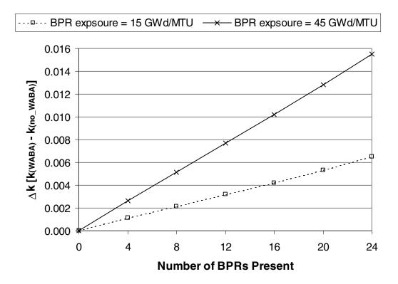
Figure 16  $\Delta k$  values for Westinghouse 17  $\times$  17 fuel with 4.0 wt %  $^{235}$ U initial enrichment and a total burnup of 45 GWd/MTU that has been exposed to various numbers of Westinghouse WABA rods for various burnup exposures
