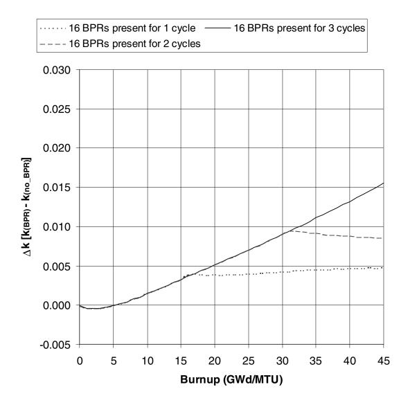
Figure 24  $\Delta k$  values as a function of burnup for B&W 15  $\times$  15 fuel with 4.0 wt %  $^{235}$ U initial enrichment that has been exposed to B&W (2.0 wt % B<sub>4</sub>C) BPRs (3 cycles of 15 GWd/MTU per cycle were assumed)
