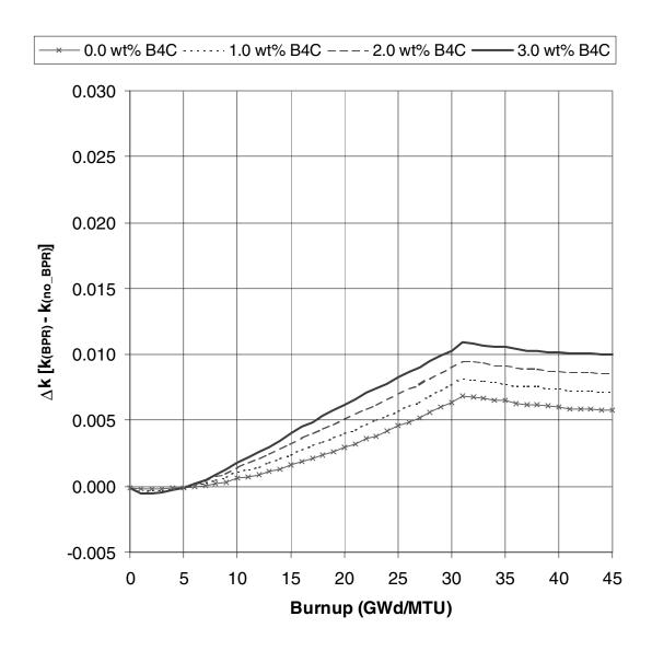
Figure 27  $\Delta k$  values as a function of burnup for B&W 15 × 15 fuel with 4.0 wt %  $^{235}$ U initial enrichment that has been exposed to B&W BPRs with varying B<sub>4</sub>C weight percents for the first 30 GWd/MTU of burnup (3 cycles of 15 GWd/MTU per cycle were assumed)
