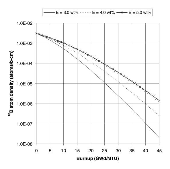
Figure 17  $^{10}$ B atom density as a function of burnup for various cases of initial fuel enrichment. The results correspond to 24 Westinghouse WABA rods inserted into Westinghouse 17  $\times$  17 fuel with various initial enrichments during the entire depletion.
