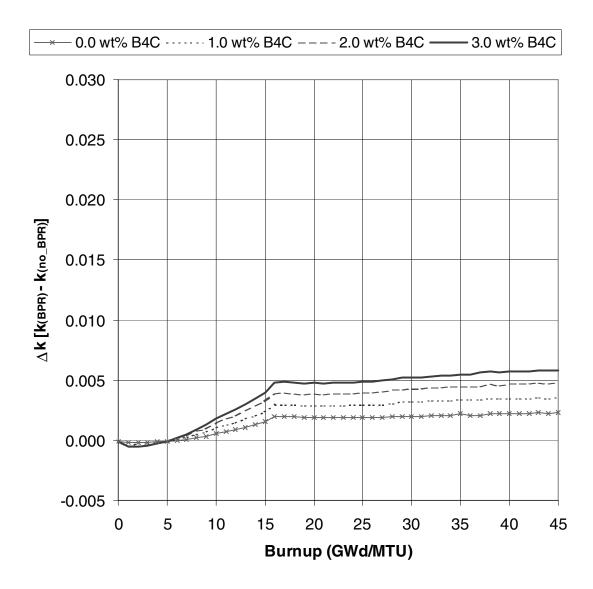
Figure 26  $\Delta k$  values as a function of burnup for B&W 15  $\times$  15 fuel with 4.0 wt %  $^{235}$ U initial enrichment that has been exposed to B&W BPRs with varying B<sub>4</sub>C weight percents for the first 15 GWd/MTU of burnup (3 cycles of 15 GWd/MTU per cycle were assumed)
