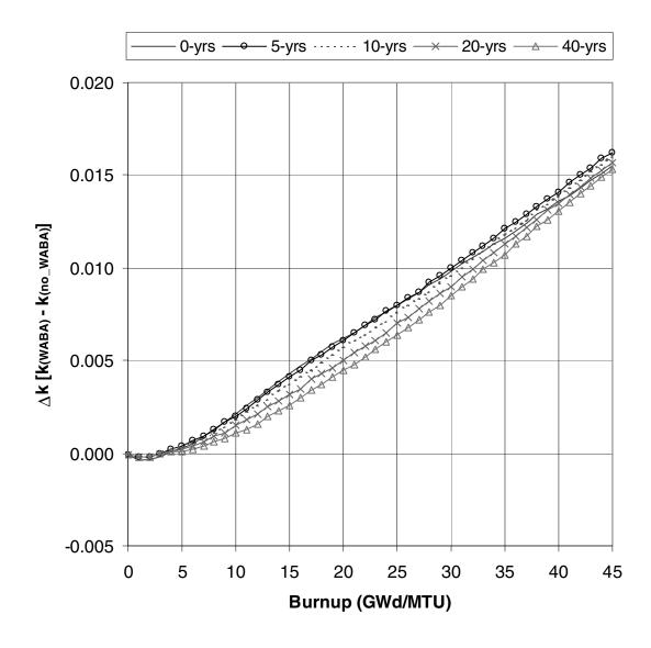
Figure 19  $\Delta k$  values as a function of burnup for various cooling times with Westinghouse 17 × 17 fuel assemblies that have been exposed to 24 WABA rods during the entire depletion (3 cycles)
