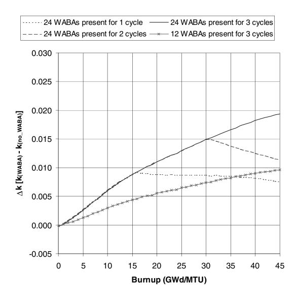
Figure 6  $\Delta k$  values as a function of burnup for Westinghouse 17  $\times$  17 fuel with 3.0 wt %  $^{235}$ U initial enrichment that has been exposed to Westinghouse WABA rods (3 cycles of 15 GWd/MTU per cycle were assumed)
