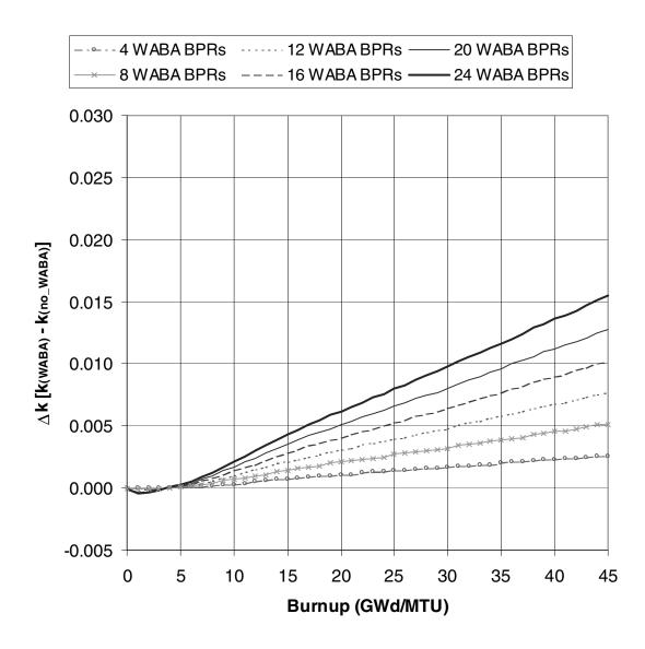
Figure 15  $\Delta k$  values as a function of burnup for Westinghouse 17  $\times$  17 fuel with 4.0 wt %  $^{235}$ U initial enrichment that has been exposed to various numbers of Westinghouse WABA rods during the entire depletion
