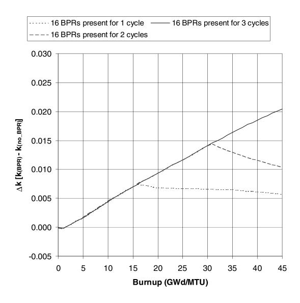
Figure 23  $\Delta k$  values as a function of burnup for B&W 15  $\times$  15 fuel with 3.0 wt %  $^{235}$ U initial enrichment that has been exposed to B&W (2.0 wt % B<sub>4</sub>C) BPRs (3 cycles of 15 GWd/MTU per cycle were assumed)
