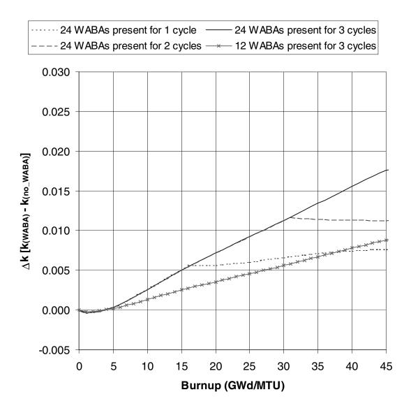
Figure 29  $\Delta k$  values as a function of burnup for Westinghouse 17  $\times$  17 fuel with 4.0 wt %  $^{235}$ U initial enrichment that has been exposed to Westinghouse WABA rods (3 cycles of 15 GWd/MTU per cycle were assumed). The results are based on SAS2H-depletion and CSAS1X-criticality calculations with "actinide + fission product" nuclides (See Table 8 for specific nuclides).
