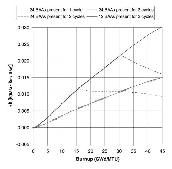
Figure 20  $\Delta k$  values as a function of burnup for Westinghouse 17  $\times$  17 fuel with 3.0 wt %  $^{235}$ U initial enrichment that has been exposed to Westinghouse Pyrex BAA rods (3 cycles of 15 GWd/MTU per cycle were assumed)
