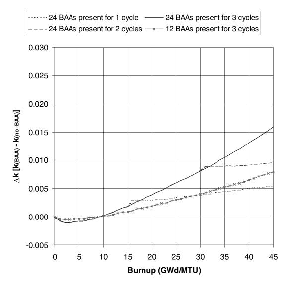
Figure 22  $\Delta k$  values as a function of burnup for Westinghouse 17  $\times$  17 fuel with 5.0 wt %  $^{235}$ U initial enrichment that has been exposed to Westinghouse Pyrex BAA rods (3 cycles of 15 GWd/MTU per cycle were assumed)
