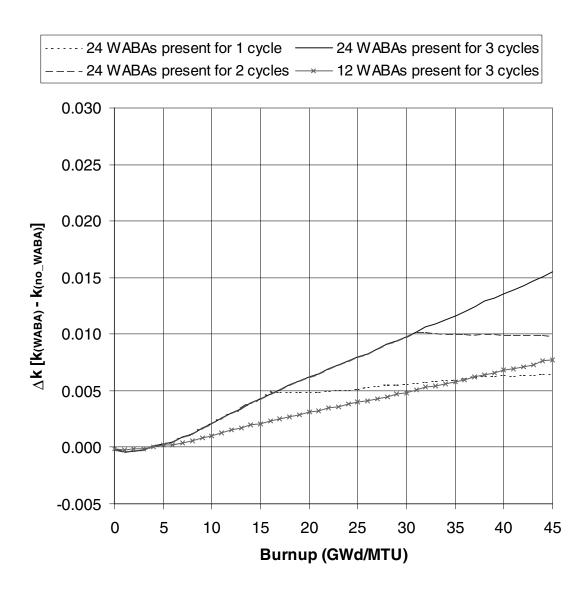
Figure 7  $\Delta k$  values as a function of burnup for Westinghouse 17  $\times$  17 fuel with 4.0 wt %  $^{235}$ U initial enrichment that has been exposed to Westinghouse WABA rods (3 cycles of 15 GWd/MTU per cycle were assumed)
