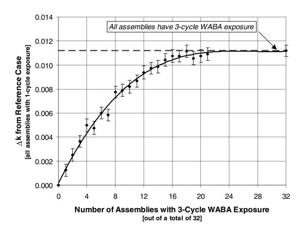
Figure 41 Increase in  $k_{\it eff}$  due to loading assemblies with 3-cycle BPR exposure into a GBC-32 cask in which the remaining assemblies have 1-cycle BPR exposure. The results correspond to Westinghouse 17  $\times$  17 fuel with 4.0 wt %  $^{235}$ U, Westinghouse WABA rods, actinide-only nuclides, and spent-fuel isotopic compositions from SAS2H depletion calculations.
