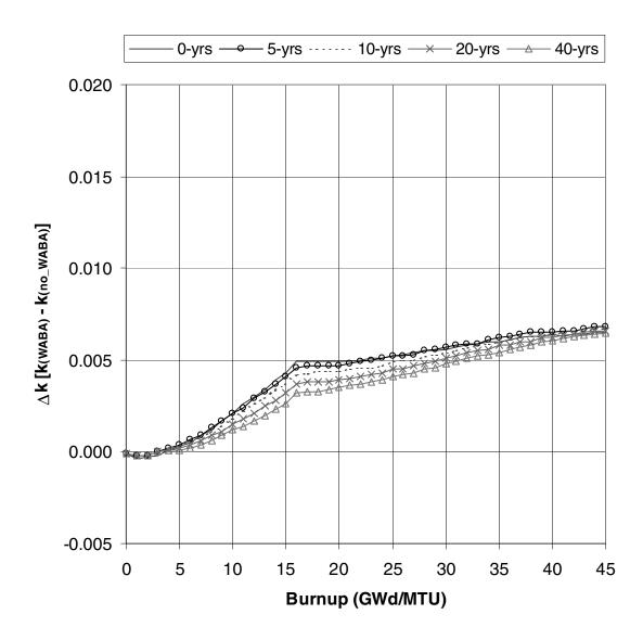
Figure 18  $\Delta k$  values as a function of burnup for various cooling times with Westinghouse 17 × 17 fuel assemblies that have been exposed to 24 WABA rods for the first 15 GWd/MTU of burnup
