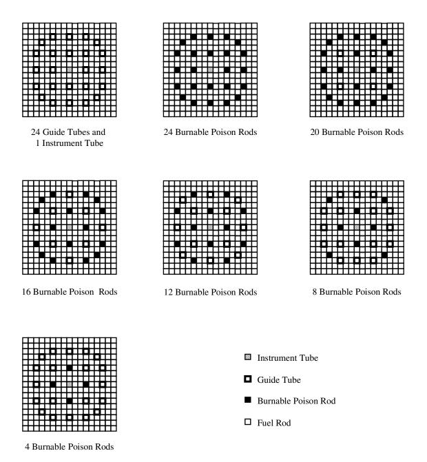
Figure 1 Pyrex BAA and WABA BPR loading patterns used for analysis (Source: Ref. 11)
