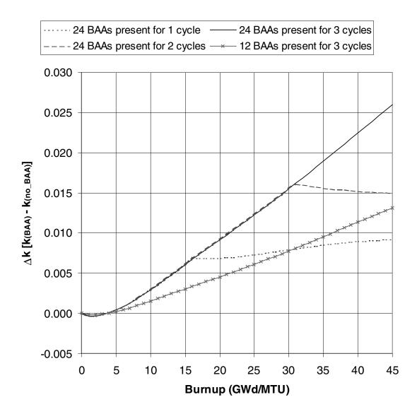
Figure 31  $\Delta k$  values as a function of burnup for Westinghouse 17  $\times$  17 fuel with 4.0 wt %  $^{235}$ U initial enrichment that has been exposed to Westinghouse BAA rods (3 cycles of 15 GWd/MTU per cycle were assumed). The results are based on SAS2H-depletion and CSAS1X-criticality calculations with "actinide + fission product" nuclides (See Table 8 for specific nuclides).
