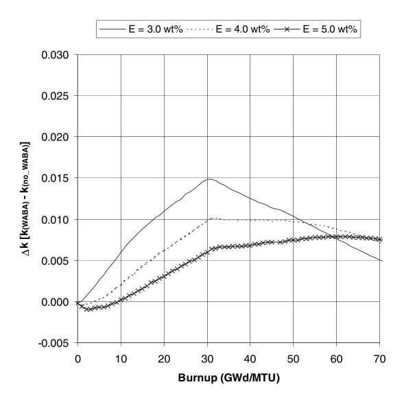
Figure 13  $\Delta k$  values as a function of burnup (for extended burnup) for Westinghouse 17  $\times$  17 fuel with various initial enrichments that have been exposed to 24 Westinghouse WABA rods for the first 30 GWd/MTU of burnup
