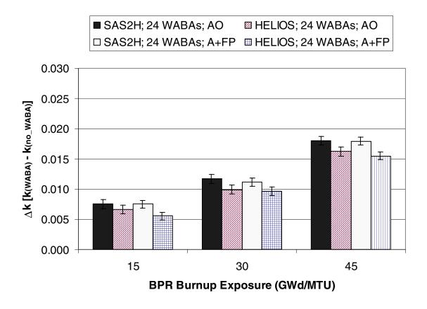
Figure 38 Comparison of reactivity differences ( $\Delta k$  values relative to the no BPR condition) in the GBC-32 cask (45 GWd/MTU, 5-year cooling) as calculated with KENO V.a for actinide-only (AO) and actinide + fission product (A + FP) burnup credit, based on isotopic compositions from SAS2H and HELIOS depletion calculations. The results correspond to fuel with 4.0 wt % <sup>235</sup>U initial enrichment that has been exposed to 24 WABA BPRs for various burnups.
