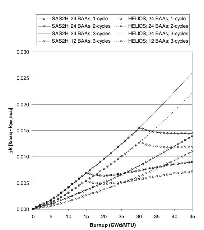
Figure 36 Comparison of reactivity differences ( $\Delta k$  values relative to the no BPR condition) as calculated with CSAS1X based on isotopics calculated with SAS2H and HELIOS for actinide-only burnup credit. The results correspond to fuel with 4.0 wt %  $^{235}$ U initial enrichment that has been exposed to either 12 or 24 BAAs.
