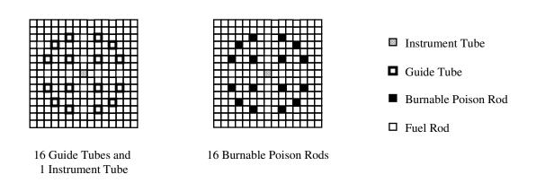
Figure 2 B&W BPR loading patterns used for analysis (Source: Ref. 16)
