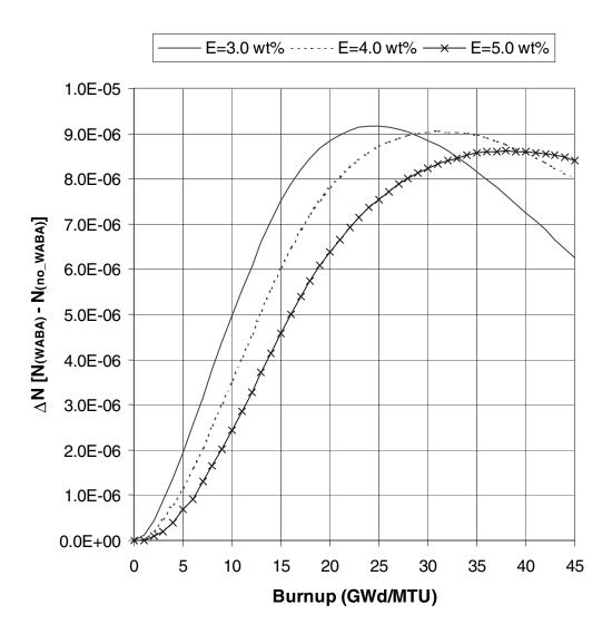
Figure 11 Differences in  $^{235}$ U atom densities,  $\Delta N$  values, as a function of burnup for Westinghouse 17  $\times$  17 fuel with various initial enrichments that have been exposed to 24 Westinghouse WABA rods for the first 15 GWd/MTU of burnup
