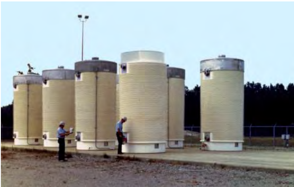
Figure 3.2-44 Castor V/21 Bolted Bare Fuel Casks
