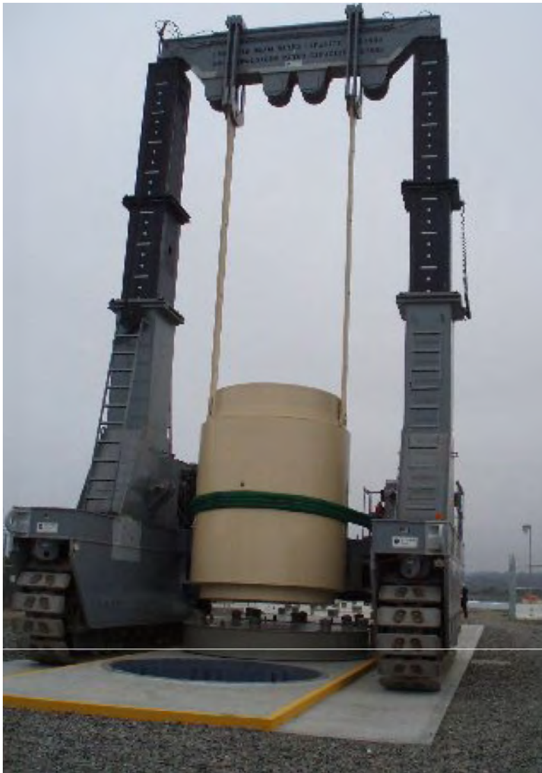
Figure 3.2-3 Holtec HI-STAR HB at the Humboldt Bay ISFSI
