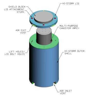
Figure 4. Typical Vertical Dry Cask-Storage System
