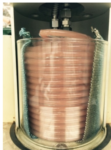
Figure 17. Quartz tube coil filled with innovative SANEX solvent and strip solution in the gamma irradiator at MFC.
