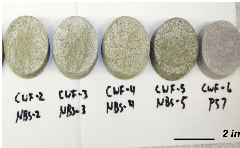
Figure 22. Photograph of ACWF samples fabricated at INL with 40% higher waste loading.
