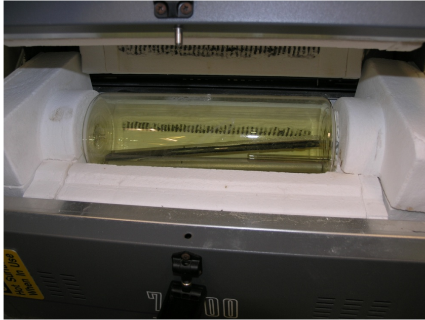
Figure 21. Photograph of Zircaloy cladding chlorination test at ORNL.
