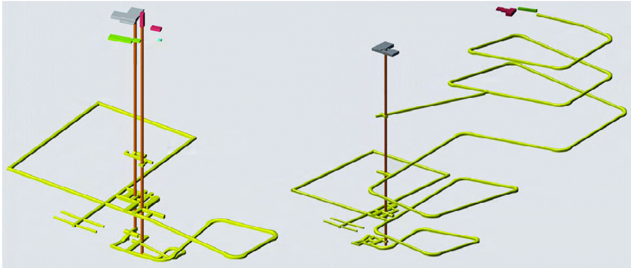
Figure 8.1. The main conceptual design alternatives for the underground rock characterization facility
