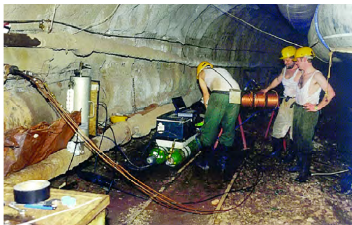
Figure 11.5. Implementation of a hydraulic test at the borehole
