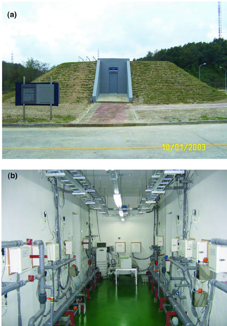
Figure 13.4. EBS test facility for near-surface disposal at KHNP/NETEC (a) Front view of engineered barrier test facility; (b) Experimental laboratory for near-surface cover performance
