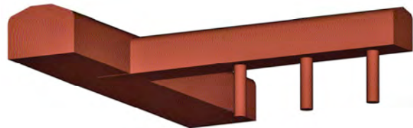
Figure 11.8. Axonometric diagram of the disposal drift arrangements
